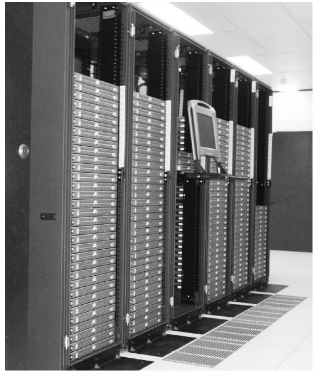
The ac3 cluster is comprised of 152 compute nodes and two head nodes, each with dual Intel® Xeon™ processors running at 3.06 GHz.
