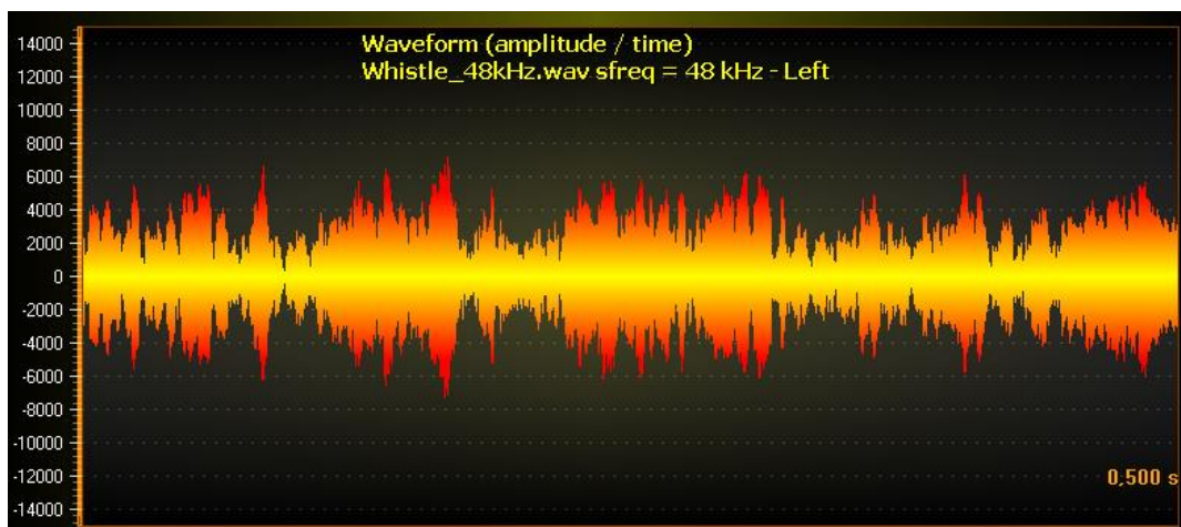
Figure 6-49. Gradient palette coloring for bipolar signal data. UsePalette for Y axis is disabled.
