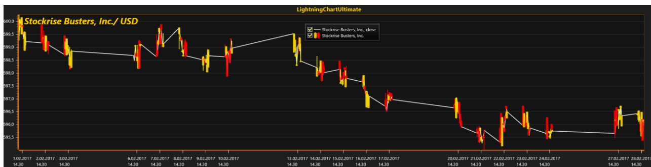
Figure 6-35. Original trading data, Monday to Friday, 10 AM – 6 PM. ScaleBreaks haven't been applied. Majority of the time range doesn't have data as stock exchange has been closed making it harder to see the essential info. PointLineSeries jumping from Close-to-Close values.
