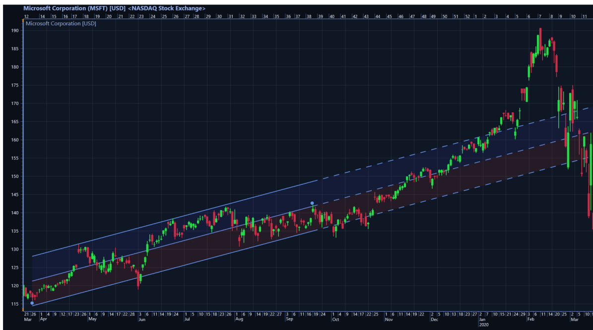
Figure 18-14. A Linear Regression Channel based on one standard deviation, ChannelType = StandardDeviations , NumberOfStandardDeviations = 1 .
