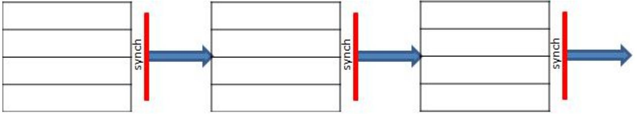
In this case cache may contain wrong data, requiring re-reading from memory. If threading is used, the number of synchronization point/barriers is more than the algorithm requires.
